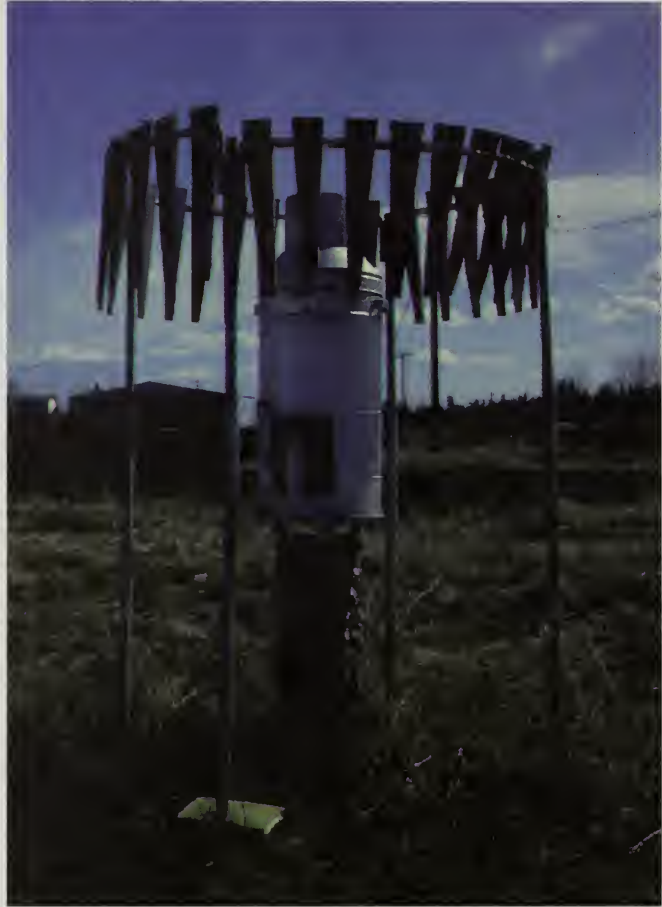
Figure 10-21 Standard rain gage altar shield
